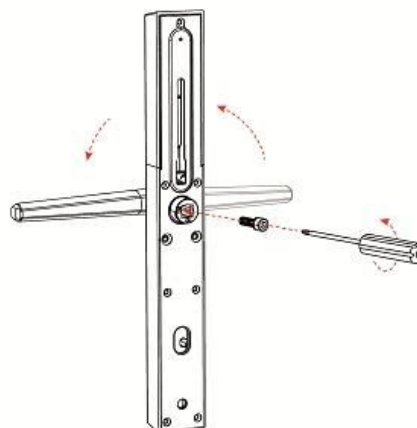
2.Adjust the direction of the handle, tighten the screws
